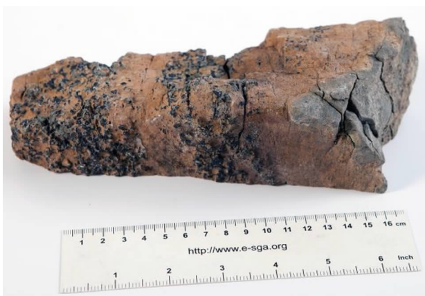
Fig.5 Sample B1b; two chromespinel layers are parallel to magnesian skarn.
