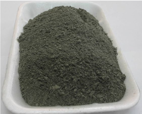
Fig.10 Cement with the addition of magnesium silicate rocks 300 m above the contact.
