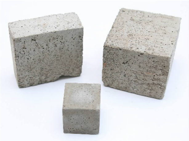
Fig.11 Samples of concrete based on magnesium silicate rocks of the Yoko-Dovyren massif.
